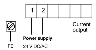
c. Power: functional extra-low voltage with safety separation (PELV) 24V DC/AC (Connection of a functional ground FE is not mandatory)
