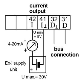
PROFIBUS-PA /FF with switching output (intrinsically safe)
