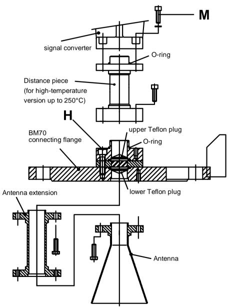
Assembly bolts for signal converter (M)
