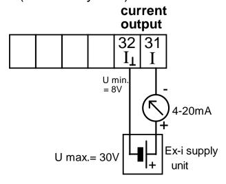
Current output HART® passive (intrinsically safe) Switching output passive (intrinsically safe)
