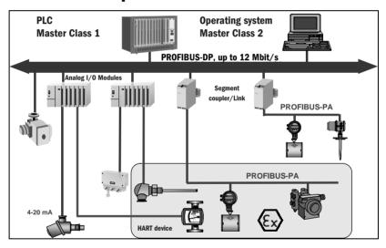
The above illustration shows a typical instrument set-up with PROFIBUS-PA devices in the hazardous and non-hazardous areas, as well as the connection of conventional non-PROFIBUS devices.
