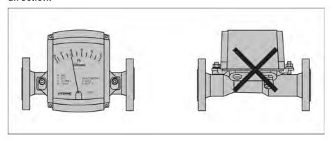
In order to comply with thermal parameters and measuring accuracy, flowmeters for horizontal installation are to be installed in the pipeline so that the display is located on the side of the measuring tube. The maximum product and ambient temperatures indicated as well as the measuring accuracy are based on lateral installation of the display.
