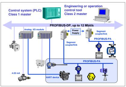
The above diagram shows a typical instrumentation with PROFIBUS-PA devices in hazardous and non-hazardous locations, including connection of conventional devices (e.g. with 4-20mA signals) to the PROFIBUS-PA. The PROFIBUS-PA is normally connected to a segment coupler which, among other things, carries out conversion to the PROFIBUS-DP. Here, it needs to be noted in particular that the segment coupler is normally set to a fixed baud rate on the DP side.
