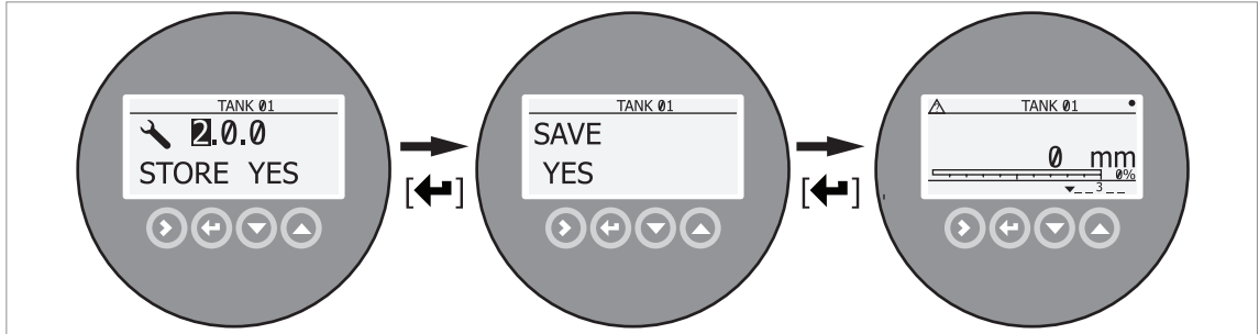
Figure 5-1: Steps to save data (WHG-approved devices)
