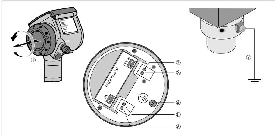
Figure 3-1: Electrical installation
