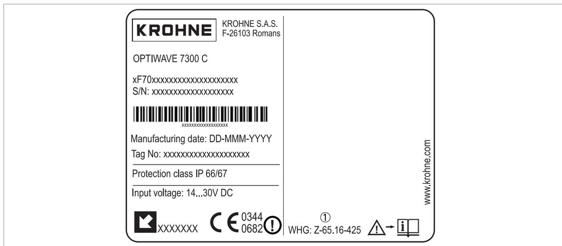
Figure 1-1: Device nameplate (device with WHG approval option)
