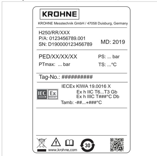
Figure 2-6: Example of a nameplate for H250 M40
