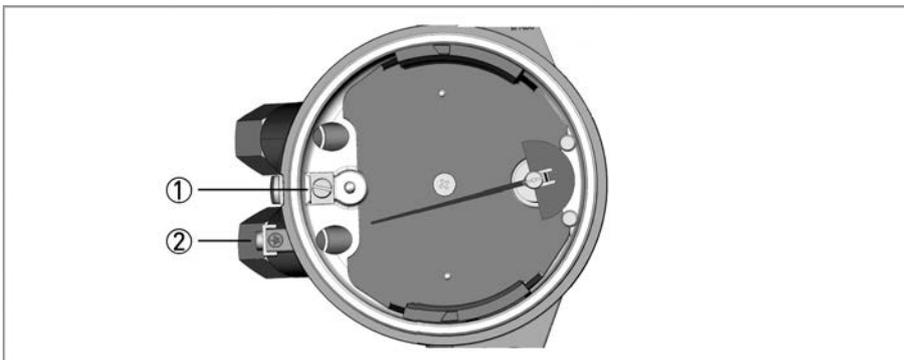
Figure 3-4: Ground terminal for H250/M40.
