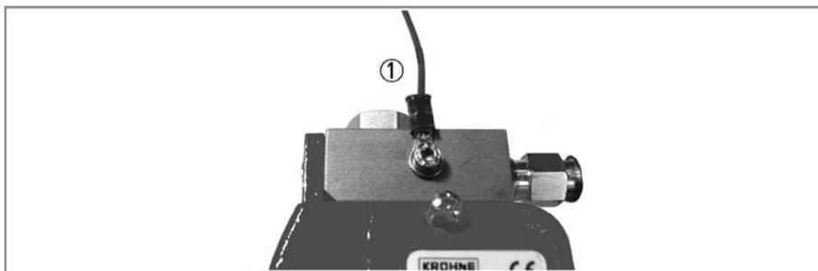
Figure 3-1: Ground terminal for DK32, DK34
