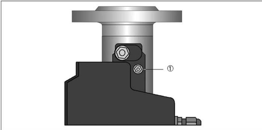
Figure 3-3: Ground terminal for H250/M8MG/.
