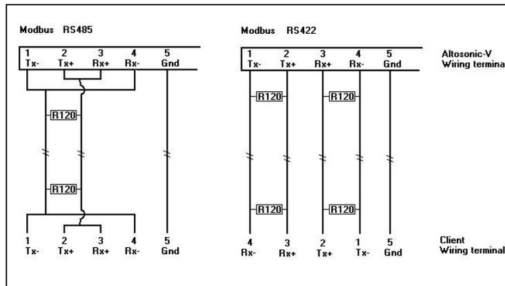
The resistors of 120 Ohm must be placed At the ALTOSONIC V wiring terminal
