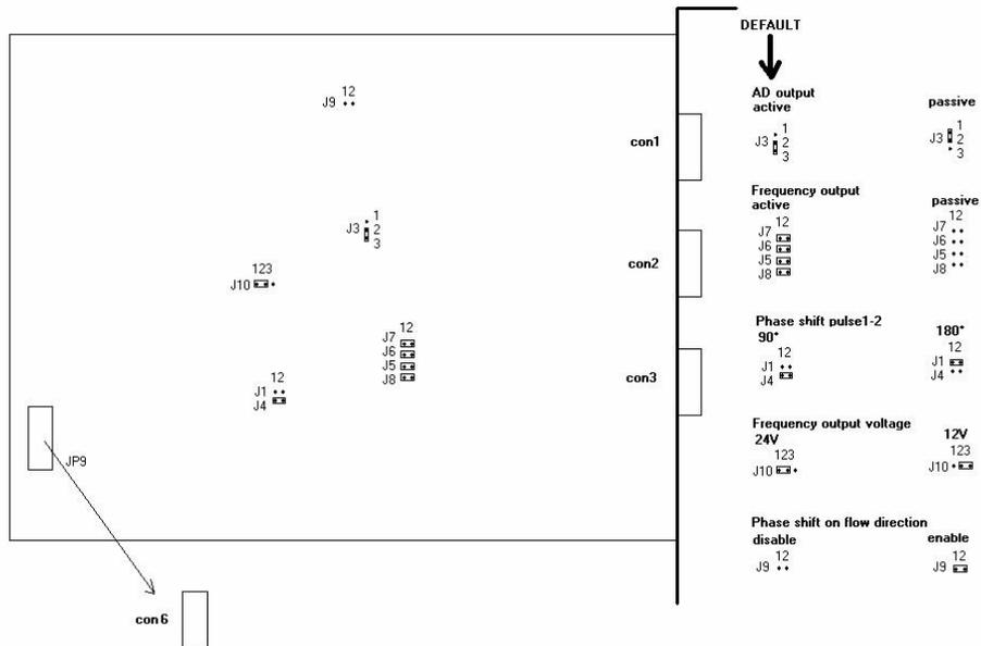
JP9 : To frequency input connector con6 (connected to frequency input bracket)
