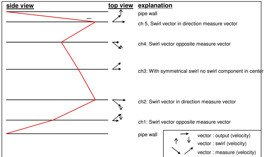
For this example in relation to normal: ch5 larger, ch1 smaller, ch4 smaller, ch2 larger, and ch3 close to normal.
