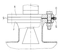
C\* = shielding strip B = BM 702 flange S\* = strap retainer F = tank flange
