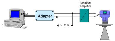
With the program PC-CAT, version 3.01 or higher, you can configurate BM 702 instruments in a very comfortable way from a PC. Connect the non-intrinsically safe side of the isolation amplifier over a load between 120  $\Omega$  and 350  $\Omega$  to the HART adapter (delivered together with PC-CAT) and connect it with a serial port of the PC.
