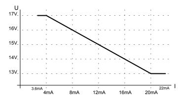
The allowed upper limit R for load+line resistance is depending on the specification of the supply unit:
