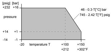
**Operating temperature** at flange <u>LP flange system:</u> -20°C (-4°F) to +130°C (302°F)
