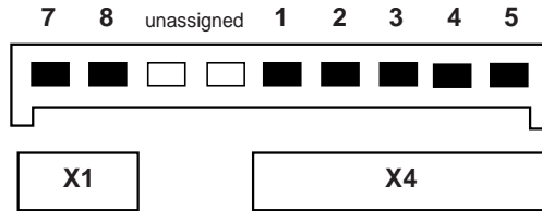
Jacks X1 and X4 on amplifier PCB, see Sect. 8.9
