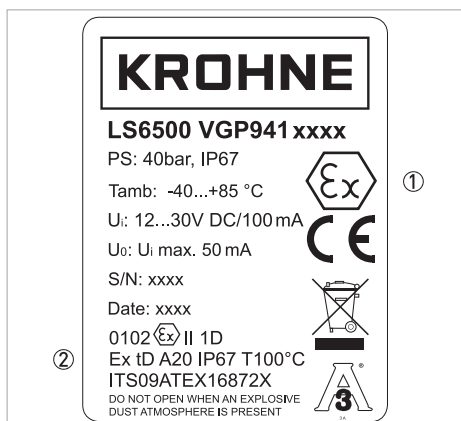
Figure 2-2: Example of Ex nameplate
