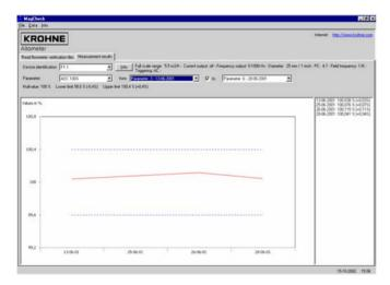
Numerical data for the related parameter are shown at the right side. Dotted lines indicate the error limits for the related parameter. These limit data are listed just above the diagram, too. In case of the first verification (no history) or selection of one verification only (e.g. from "Parameter 6" to "Parameter 6" results are shown as numerical values.
