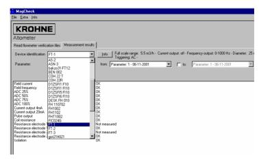
Pull-down lists will allow selection of a sequence of meter verifications in the meter history. As an example the following view shows meter FT-1, parameter "ADC 100%" for verifications 3 to 6 out of a sequence 1 to 7. Any other parameter may be presented in the same way.
