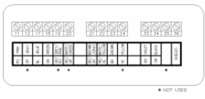
Fig. 30: Converter terminal box connections
