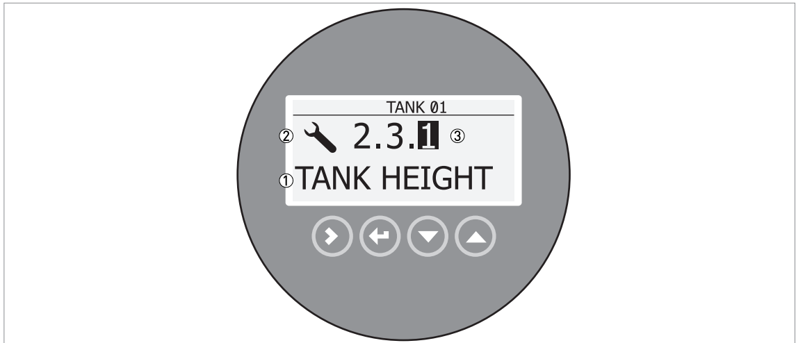
Figure 5-2: Local display screen layout in configuration mode
