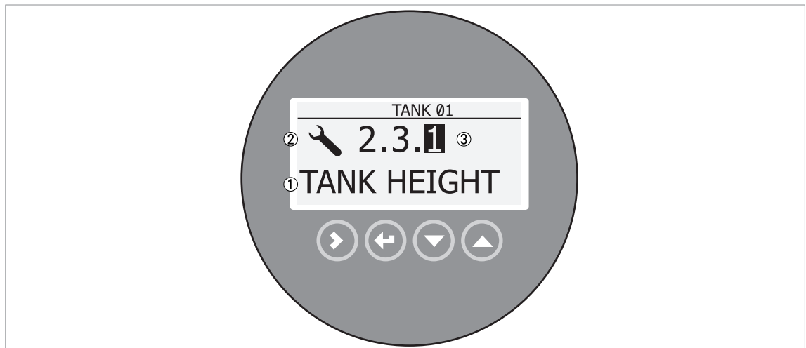
Figure 6-1: Local display screen layout in configuration mode
