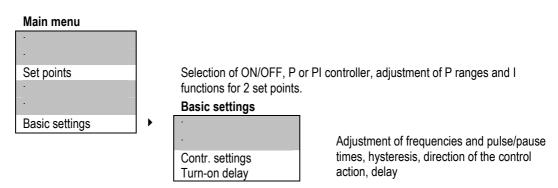
For any type of controller you have to enter one or two set points, and you have to tell the device whether these set points are reached by increasing or decreasing the measured value.
