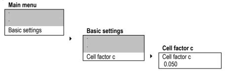
Please make sure that the cell factor of the sensor is appropriate for the selected measuring range. In contrast to the device which can be used for all ranges, the sensor's applicability is limited by its geometrical design, i. e. the size and arrangement of its electrodes. The cell factor is the numerical expression of this design. With this cell factor the device can process the measurement and calculate standardized conductivity values.
