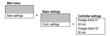
In the basic settings of the controller you can define, how long a controller is supposed to dose with 100% without raising alarm.
