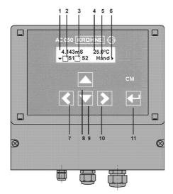
1 Measured value 2 Status relay 1 3 Status relay 2 relay OFF relay ON 4 Temperature 5 Controller AUTO: controller ON MAN: controller OFF (manual operation of the relays) 6 Orientation aids 7 Kev left ( ◀ ) 8 Key up ( • ) 9 Key down (▼) 10 Key right ( ▶ ) 11 Key "Enter"
