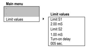
For the alarm, you can adjust two limits:
