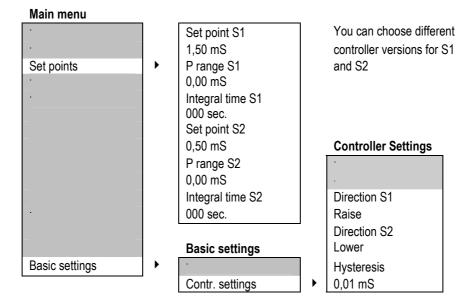
For an ON/OFF controller you have to set the following parameters:
