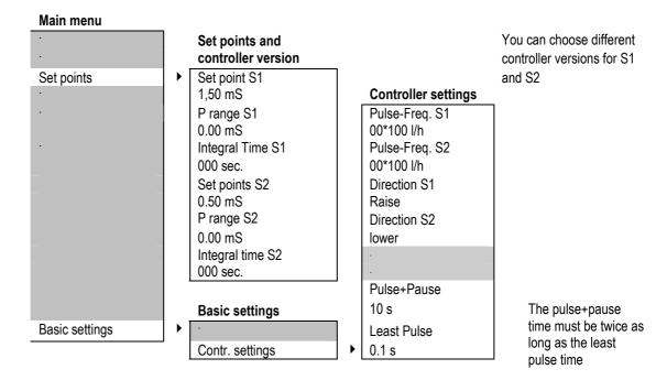
For a pulse-pause controller you have to set the following parameters:
