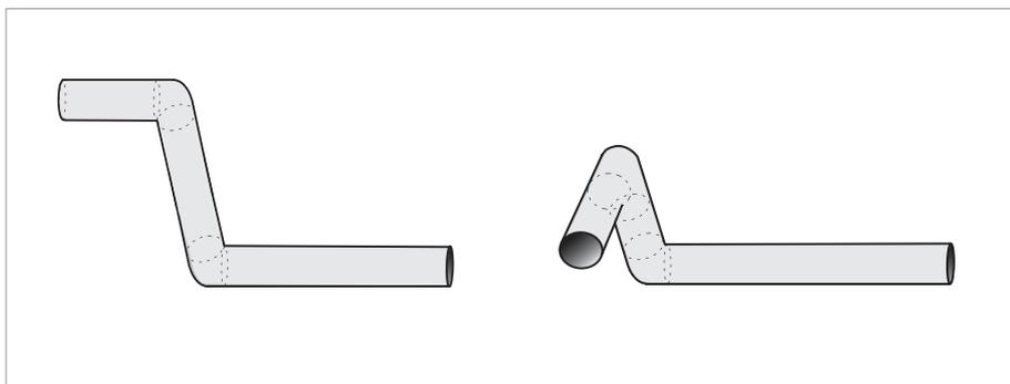
Figura 3-4: 2 and 3 dimensional bends, in front of flowmeter
