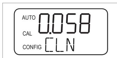
A message of a calibration error, i.e. the calibration is deficient, differs from the other error messages and looks like the following:
