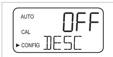
If you enabled the desiccant alarm and the humidity detector determines a problematic value, the device activates the alarms and sets the 4...20 mA output to the selected error level. In the normal measuring mode you see the measured value in the upper row and "DESC" in the lower row:
