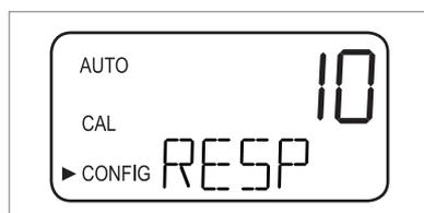
With the help of this function you can adjust the speed of response for both the displayed NTU/FNU value and the output values (i.e. of the RS 485 or the 4...20 mA output). The default setting is 10, the adjustable range is 1...100.
