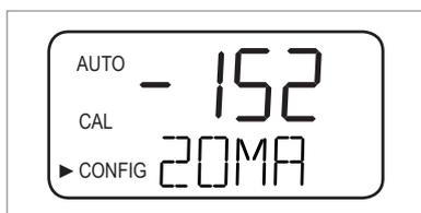
After accepting the adjustment for the 20 mA output by pressing  $\leftarrow$  the device switches back to the normal measuring mode (AUTO). All settings are saved.
