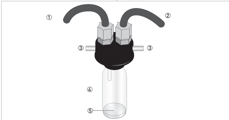
Figure 2-3: Description of ultrasonic cuvette with flow-through holder
