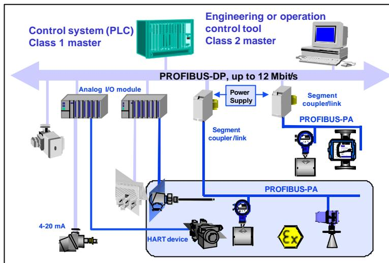
The diagram above shows a typical instrumentation with PROFIBUS-PA devices in hazardous and non-hazardous locations, including connections of conventional devices (e.g. with 4-20mA signals) to the PROFIBUS-PA.
