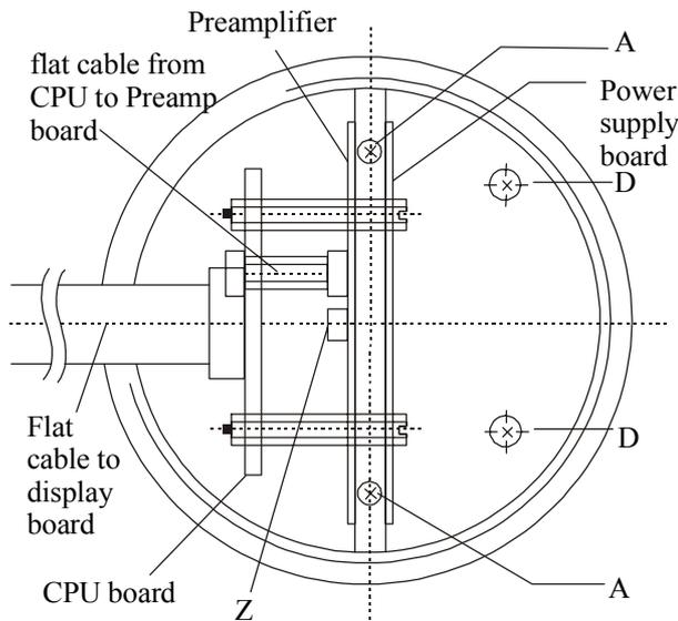
2. Remove screws **A** and turn display board to one side.
