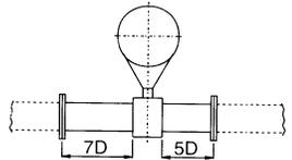
With flow straightener the inlet pipe length may be halved e.g. for a control valve the inlet length is 25D instead of 50D. The minimum inlet pipe length including flow straightener must always be 12 D. The small sizes (below 1" or DN 25) come with upstream & downstream pipelines & flange connections to suit customer's flanges.
