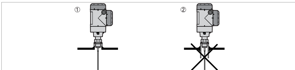
Figure 2-14: Sockets for threaded process connections
