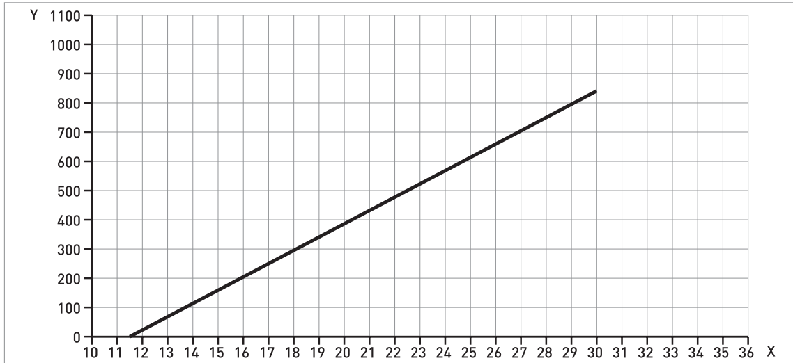
Figure 3-8: Minimum power supply voltage for an output of 22 mA at the terminal (Non-Ex and Hazardous Location approval (Ex i / IS))
