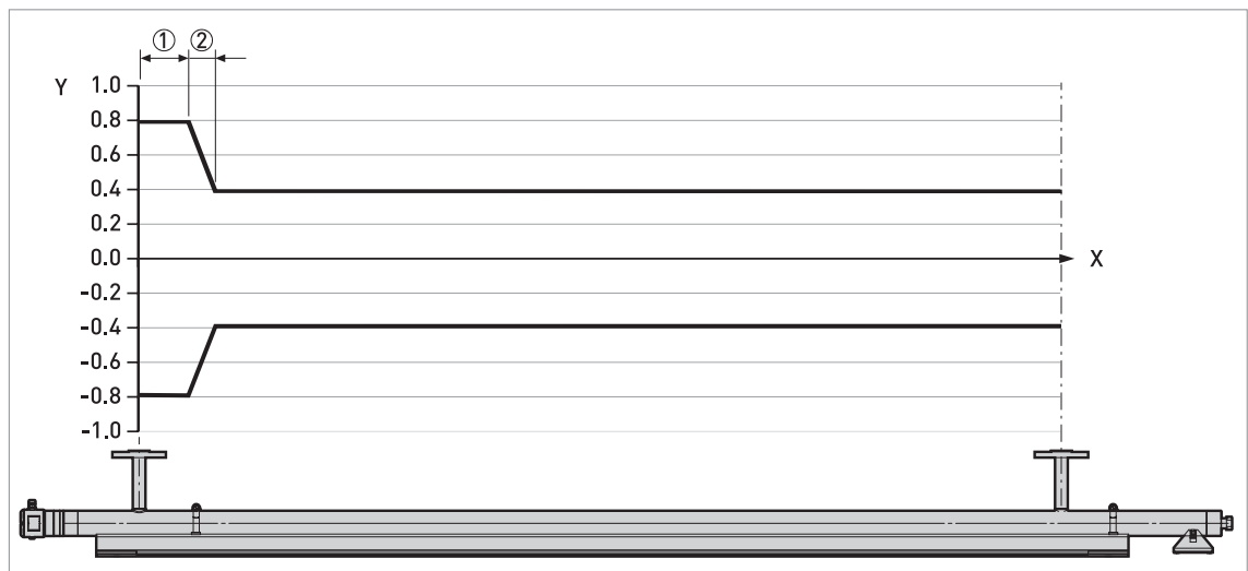
Figure 5-2: Measuring accuracy / distance from the process connections of the bypass chamber, in inches
