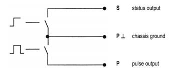
The pulse and status outputs can be operated in the active or passive mode.
