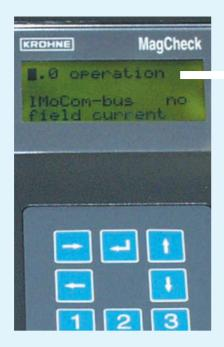
MagCheck lets you check electromagnetic flowmeters (KROHNE EMFs) periodically for proper and accurate functioning. This allows you to meet your in-house regulations e.g. based on ISO 9000, or official requirements easily and at low cost.
