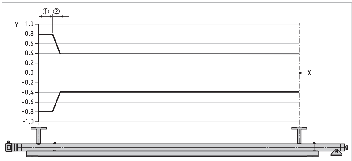
Figure 2-2: Measuring accuracy / distance from the process connections of the bypass chamber, in inches
