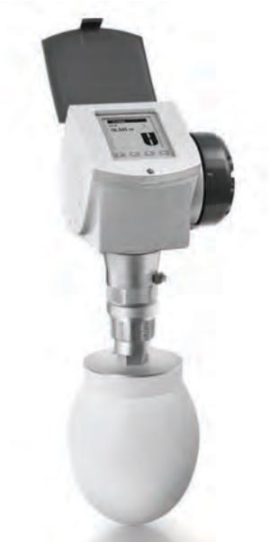
Drop antennas are a unique innovation to measure powders and other solids in very dusty atmospheres. The ellipsoidal shape of the antennas prevents build-up and generates a small beam angle for accurate measurement of silo contents. They have these features:
