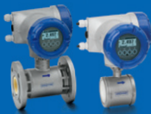
OPTIFLUX 7000 EMF with capacitive electrodes that do not come in contact with the media are designed for applications that use adhering media and liquids with low conductivity levels. Stable measurements even in noisy applications.
