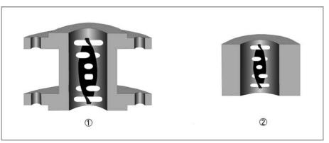
Figure 3-3: Types of magnetic filters
