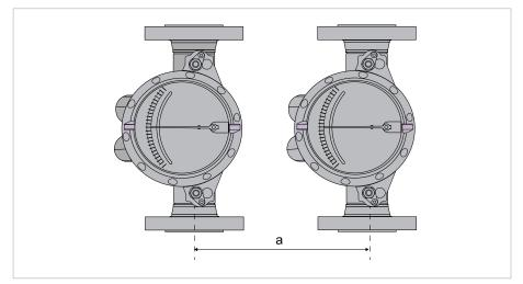
Figure 3-1: Minimum distance between devices
