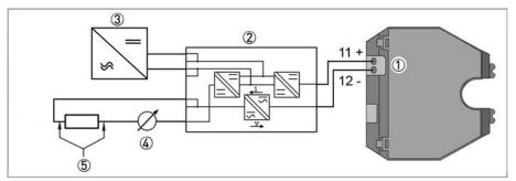
Figure 4-7: Power supply of ESK4A with galvanic isolation
