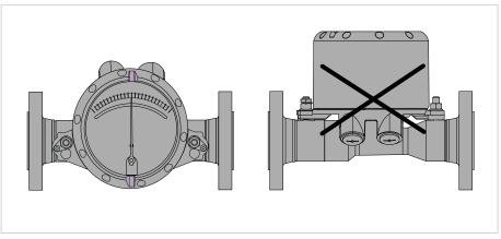
Figure 3-2: Installation position for H250H
