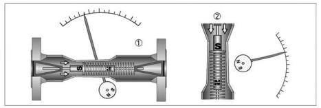
Figure 8-2: Measuring principle for H250H and H250U
