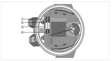
Figure 4-8: Position of the connection terminals
