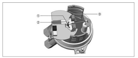
Figure 7-2: Retrofitting of the limit switch
