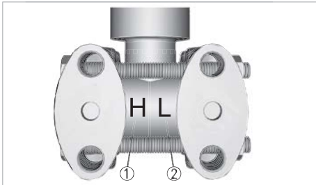
Figure 3-3: Process connection of the differential pressure transmitter
