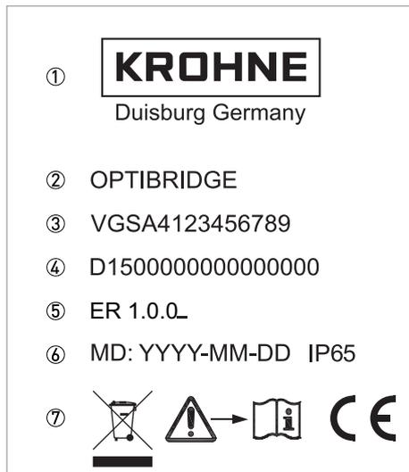
Figure 2-3: Example for a nameplate
