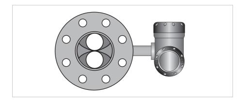
The meter can be installed with the converter (or remote junction box) on the side of the meter so that the measuring tubes are sitting one above the other. Avoid this method of installation where there is a two phase process flow, or where the process fluid contains gas. If this situation cannot be avoided, please contact the manufacturer for advice.
