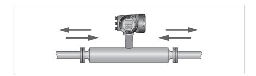
Mass flowmeters have a maximum level of force (negative or positive) that can be applied to the ends of the meter. Refer to the table in the technical data section of this Handbook for the maximum end loadings.
