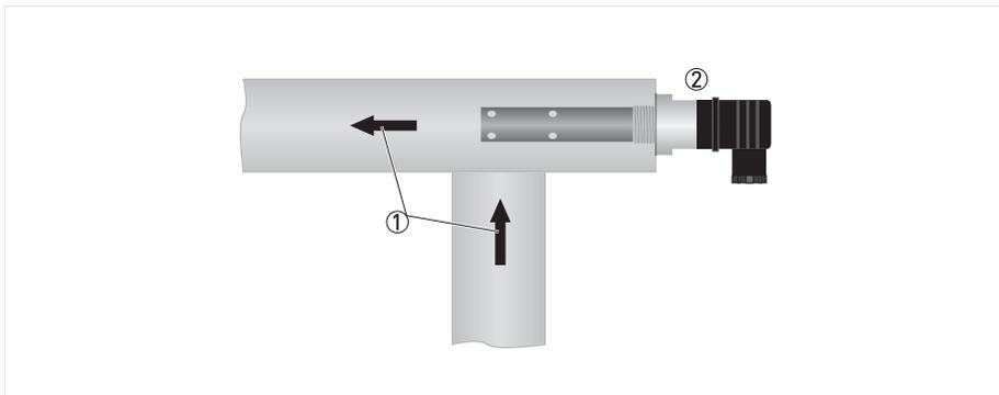
Figure 3-6: Installation for clean water
