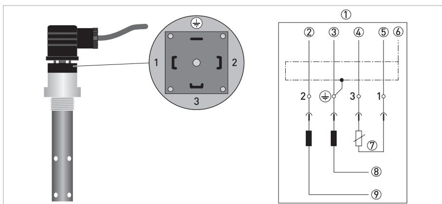
Figure 3-2: Cable assign of a Hirschmann plug
