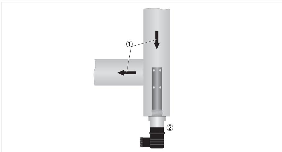
Figure 3-5: Installation for clean water
