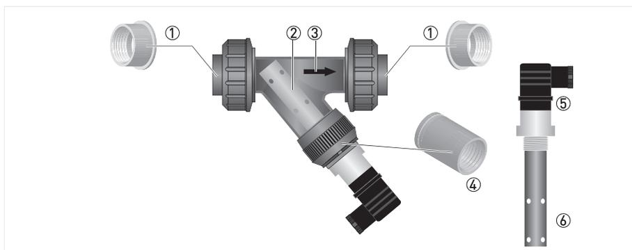
Figure 3-10: Installing the sensor into the flow-through assembly
