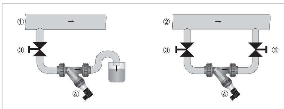
Figure 3-9: Possible mounting positions of the flow-through assembly
