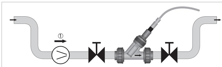
Figure 3-3: Installation requirements for the sensor
