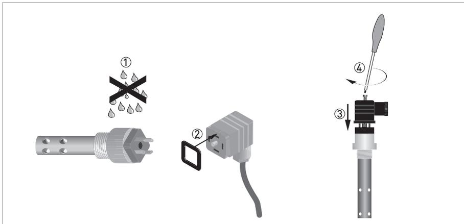
Figure 3-1: Connecting the Hirschmann plug to the sensor
