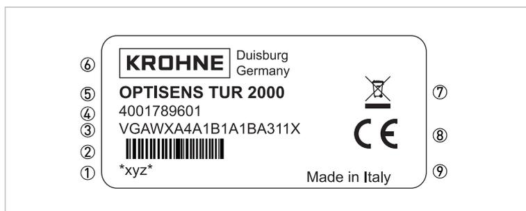
Figure 2-3: Example for a nameplate
