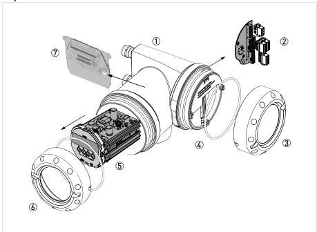
Figure 7-2: Disassembled compact device
