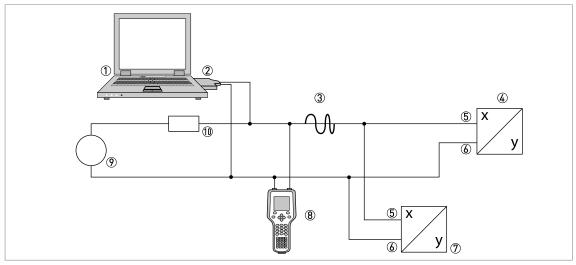
Figure 9-2: Multi-Drop connection (2-wire connection)
