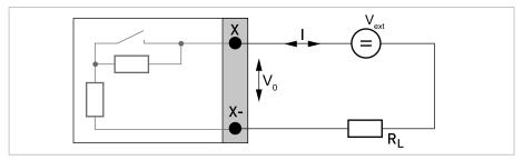
Figure 4-26: Pulse/frequency output passive  $P_N$  according to IEC 60947-5-6 (NAMUR) Ex i
