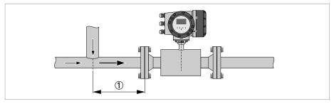
Figure 3-5: Distance behind a T-section
