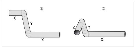
Figure 3-4: 2 and/or 3 dimensional bends upstream of the flowmeter
