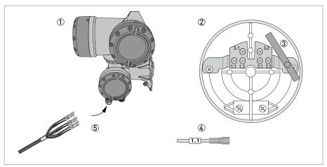
Figure 4-2: Construction of field version
