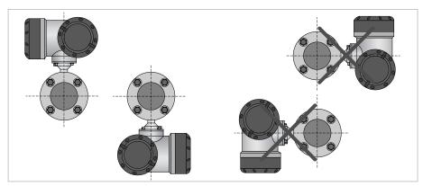
Figure 3-13: Installation position on horizontal pipe sections
