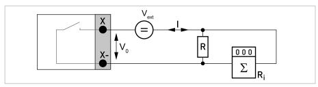
Figure 4-16: Pulse/frequency output passive Pp
