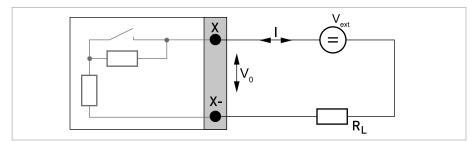
Figure 4-27: Status output / limit switch  $S_{N}$  according to IEC 60947-5-6 (NAMUR) Ex i
