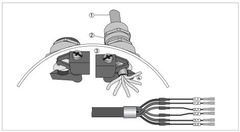
Figure 4-3: Clamp the cables on the shielding bush
