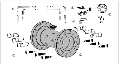
Figure 7-1: Disassembled device, remote (field) version
