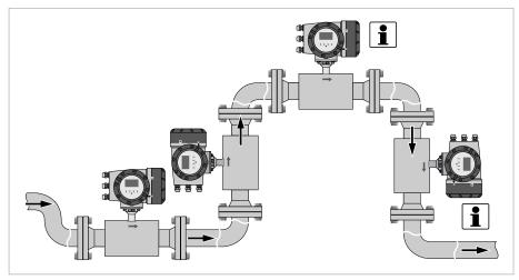
Figure 3-6: Installation in bending pipes (90°)
