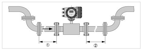
Figure 3-3: Recommended inlet and outlet
