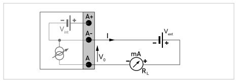
Figure 4-9: Current output passive  $I_p$
