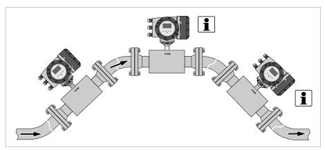
Figure 3-7: Installation in bending pipes (45°)
