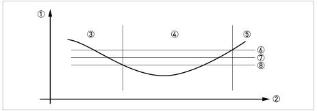
Figure 6-8: Indication of low flow cutoff
