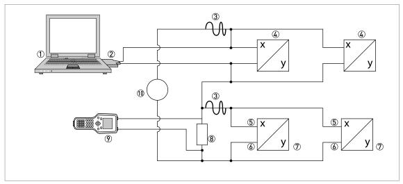
Figure 9-3: Multi-Drop connection (3-wire connection)
