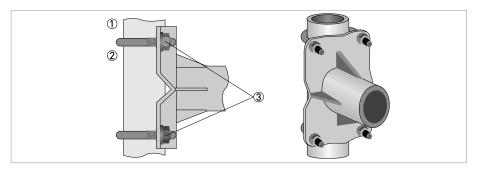
Figure 3-14: Pipe mounting of the field housing
