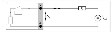
Figure 4-20: Status output / limit switch  $\rm S_{N}$  according to IEC 60947-5-6 (NAMUR)
