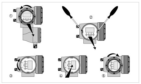
Figure 3-15: Turning the display of the field housing version
