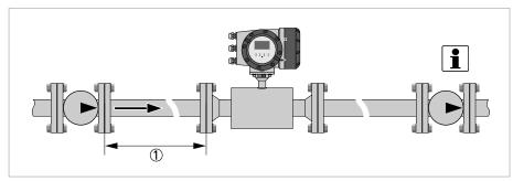
Figure 3-8: Installation behind a pump
