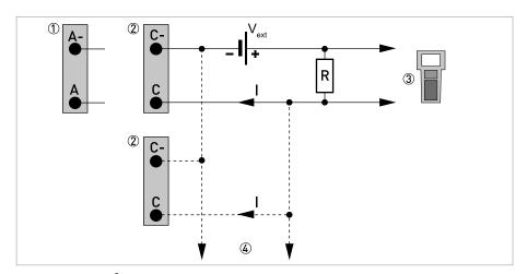
Figure 4-30: HART® connection passive (Ip)
