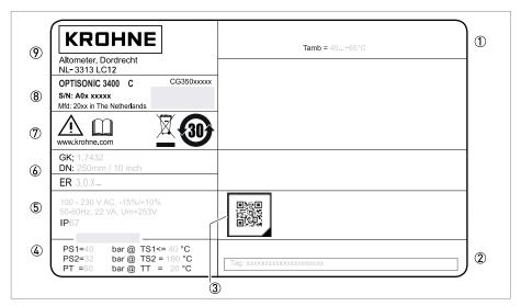
Figure 2-4: Example of nameplate for the compact version
