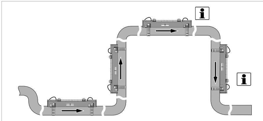
Figure 3-6: Mounting on vertical pipelines is possible
