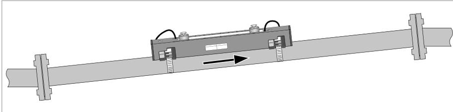
Figure 3-2: Install on a slightly ascending pipe section
