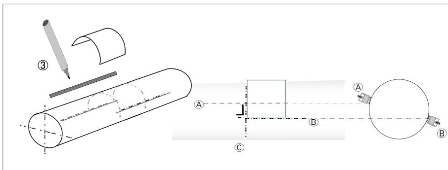
Figure 3-18: Markings on the pipeline
