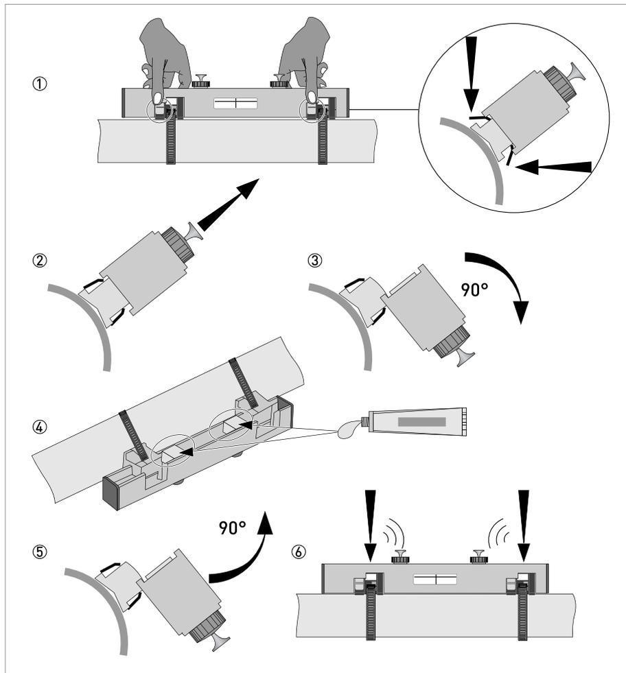
Figure 3-20: Greasing transducers
