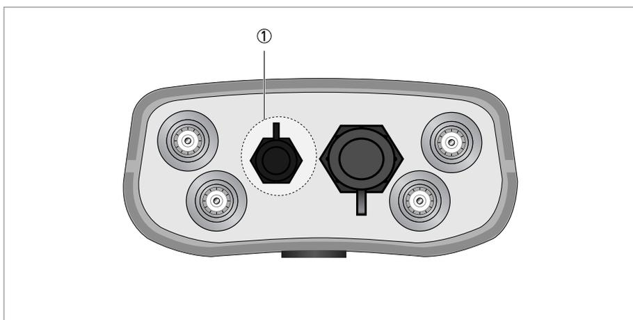
Figure 5-1: ① Connection 12 VDC power supply input
