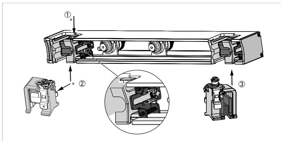
Figure 3-19: Installing magnetic fixation units
