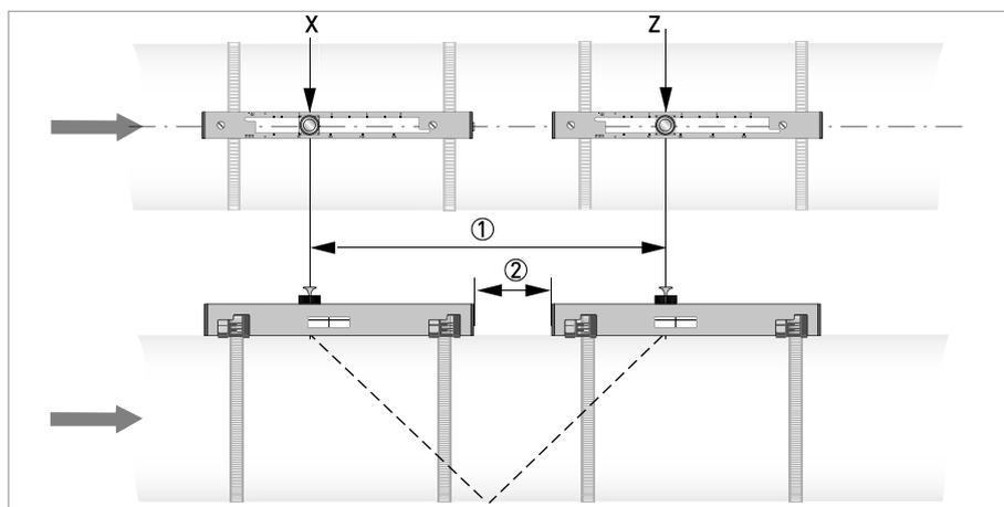
Figure 3-13: Mounting 2 rails in V-mode (2 traverses)
