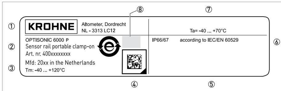
Figure 2-3: Example of a flow sensor nameplate
