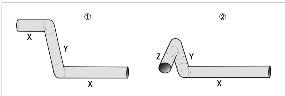
Figure 3-3: 2 and/or 3 dimensional bends upstream of the flowmeter
