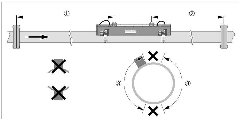
Figure 3-1: Inlet, outlet and recommended mounting area
