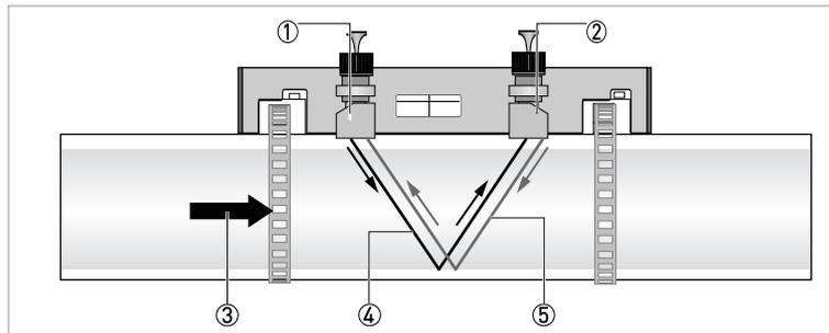
Figure 7-1: Measuring principle (example reflected path set-up)
