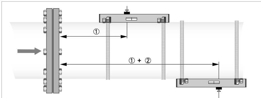
Figure 3-14: Mounting second rail in Z mode (1 traverse) using a reference point
