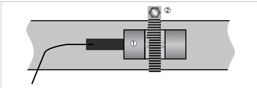
Figure 4-2: Mounting PT 100 with hose clamp
