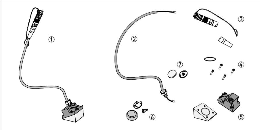
Figure 6-2: Disassembled transducer cable
