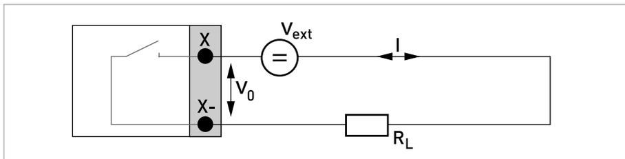
Figure 5-8: Status output / limit switch passive  $S_p$ **Current input active**
