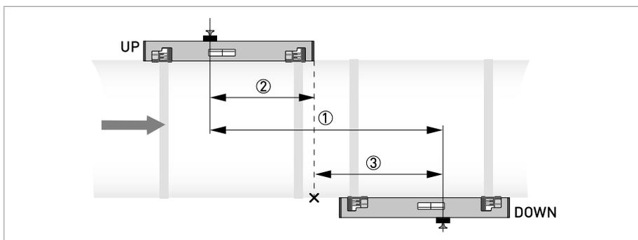
Figure 3-15: Mounting second rail in Z mode (1 traverse) without using a reference point
