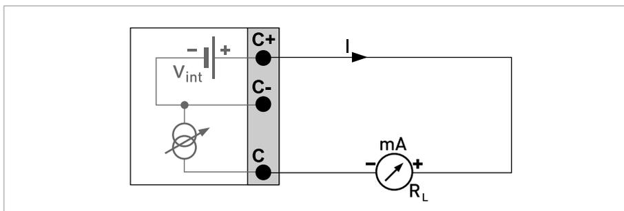
Figure 5-4: Current output active  $I_a$ **Current output passive, basic I/Os**
