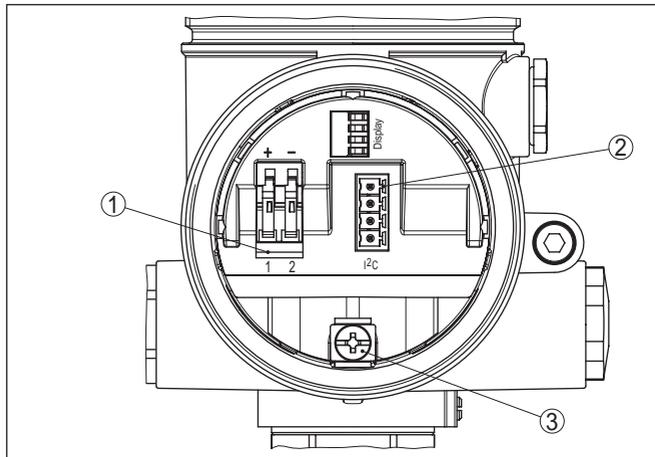
Fig. 21: Connection compartment, double chamber housing
