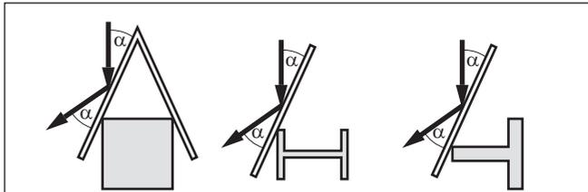
Fig. 11: Cover flat, large-area profiles with deflectors
