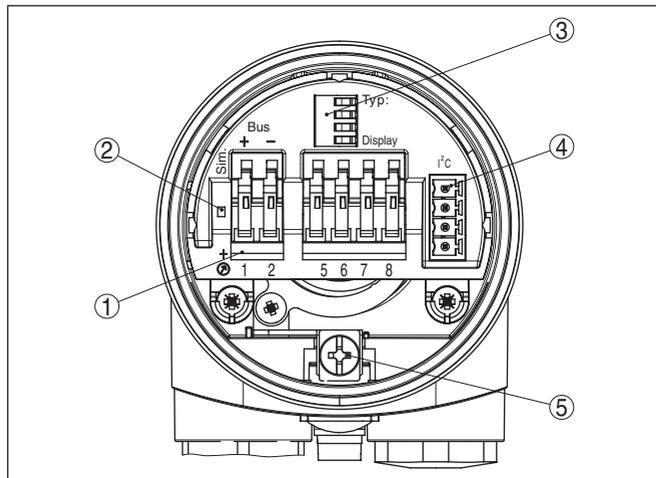
Fig. 17: Electronics and connection compartment - single chamber housing
