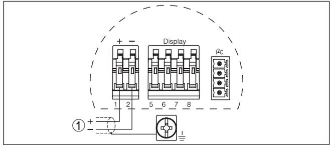
Fig. 18: Wiring plan - single chamber housing
