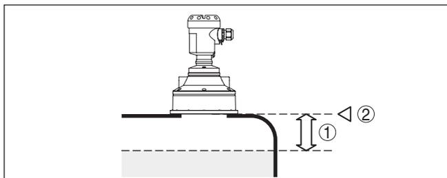
Fig. 3: Minimum distance to the max. level
