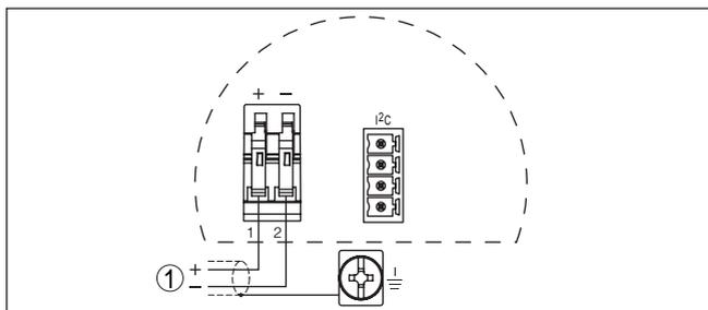
Fig. 22: Wiring plan - double chamber housing
