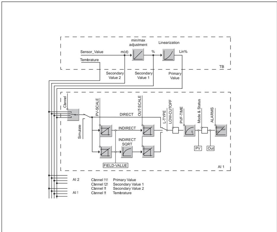
Fig. 27: OPTISOUND 3030 C measured value processing
