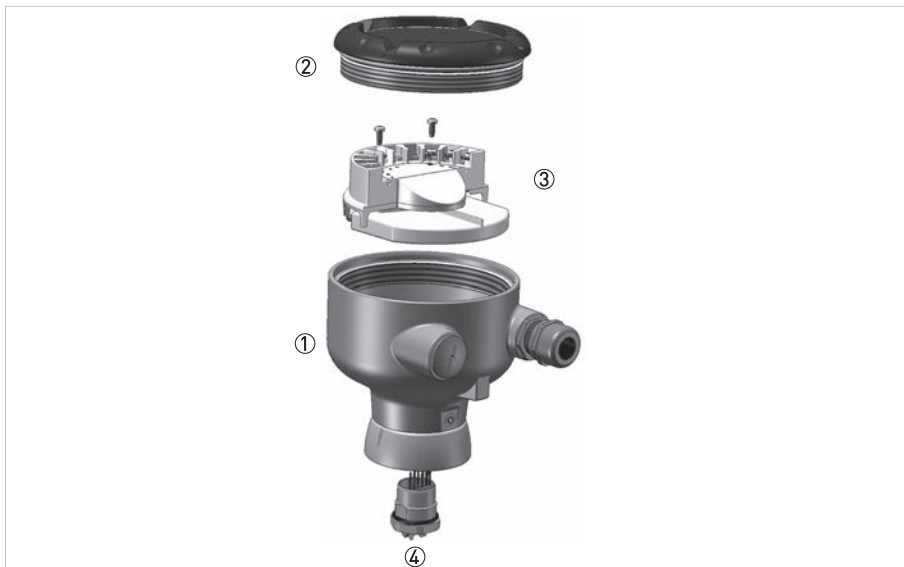
Figure 7-5: Exploded view of remote sensor connection box
