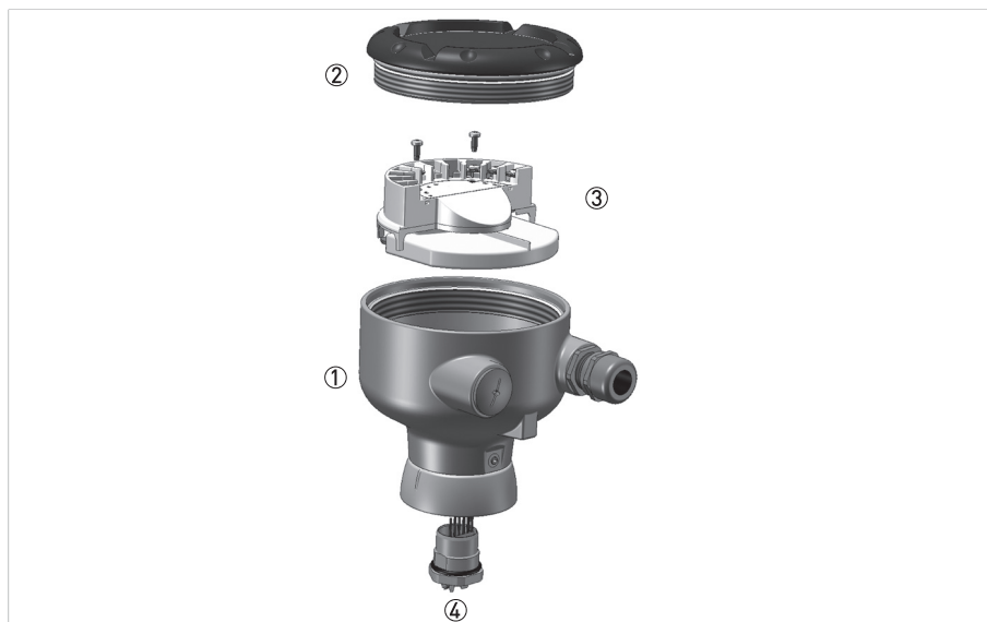
Figure 7-5: Exploded view of remote sensor connection box
