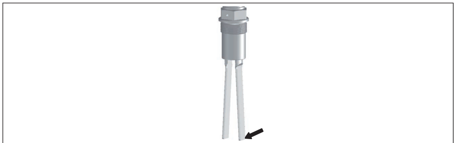
Fig. 13: Max. lateral load alongside fork side (narrow fork side)
