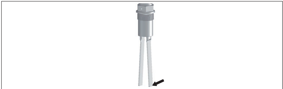
Fig. 15: Max. lateral load alongside fork side (narrow fork side)
