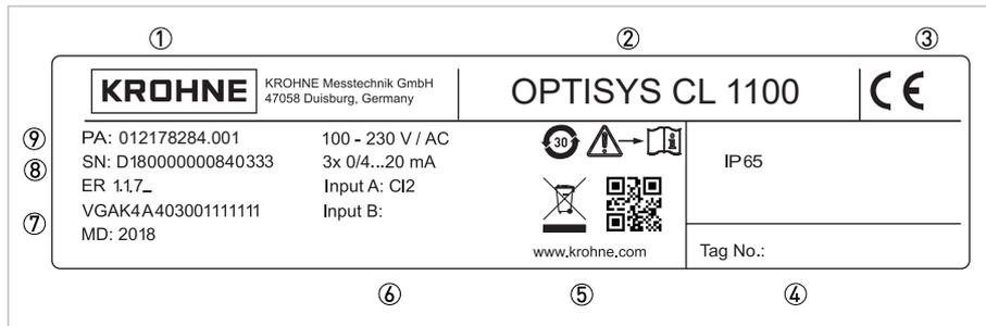
Figure 2-5: Example for a nameplate
