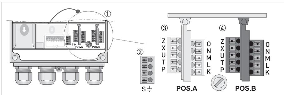
Figure 4-2: Sensor connection terminals on the signal converter
