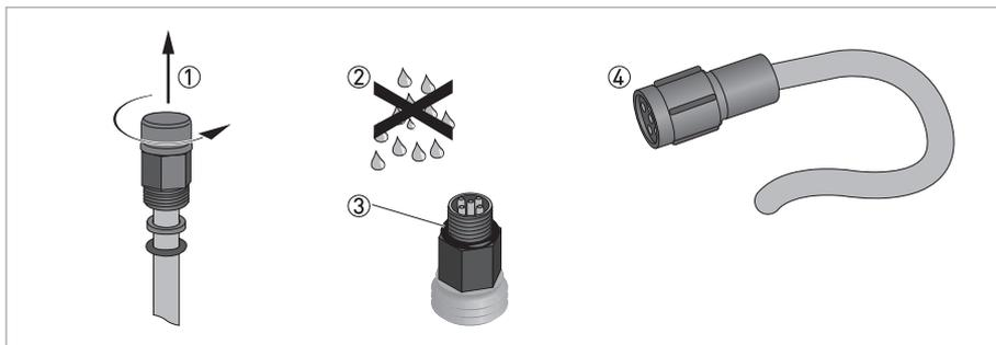
Figure 4-1: Connecting the cable to the sensor
