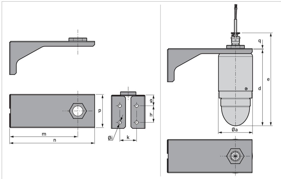
Figure 8-10: Device with a wall-mounted bracket
