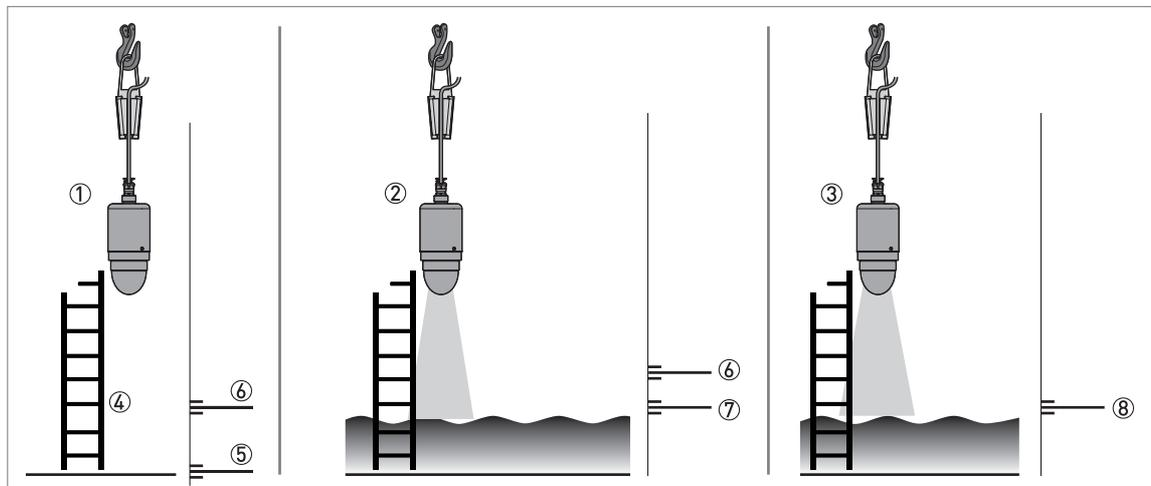
Figure 6-5: How to make a filter to remove radar signal interference
