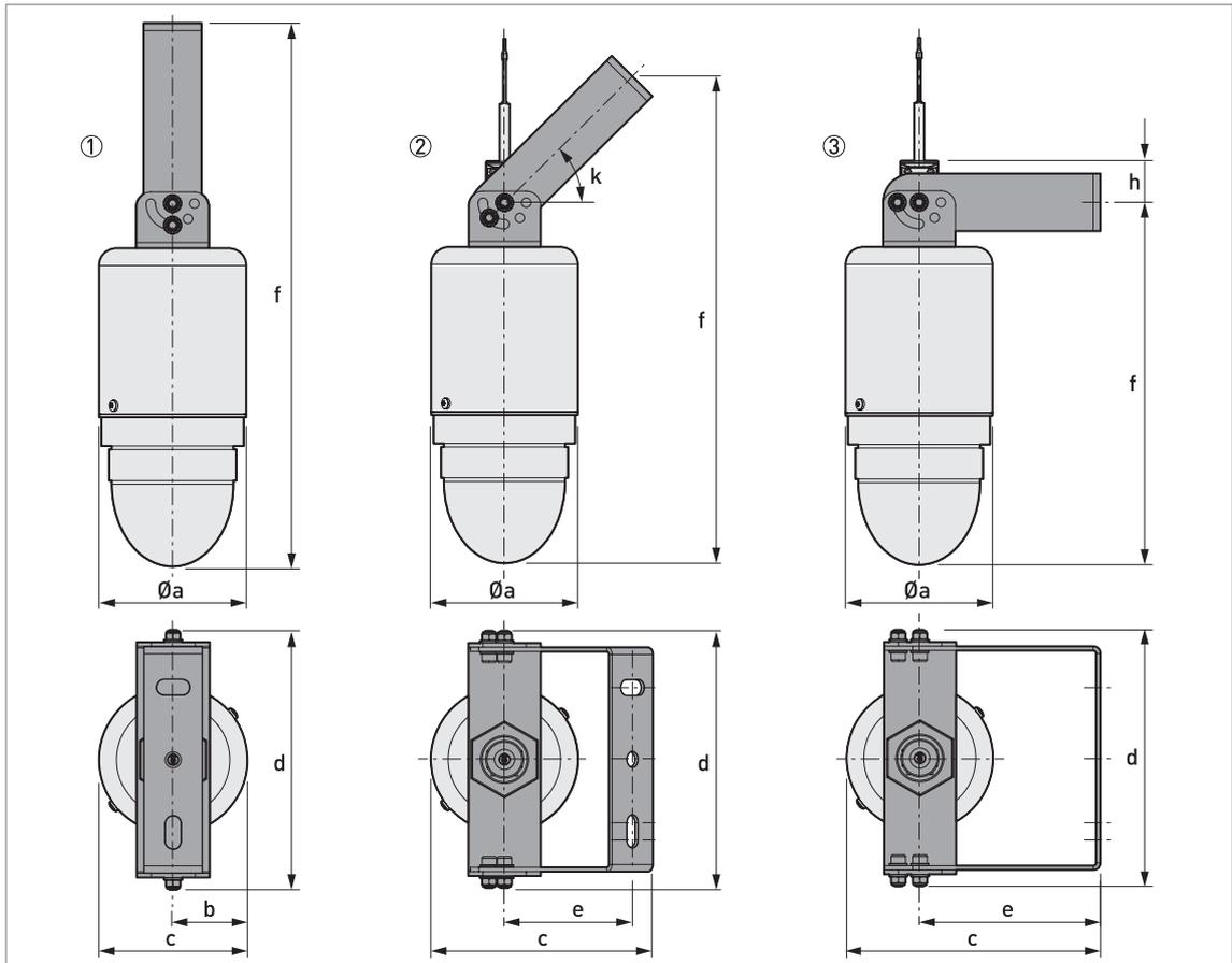
Figure 8-8: Device with an orientable bracket
