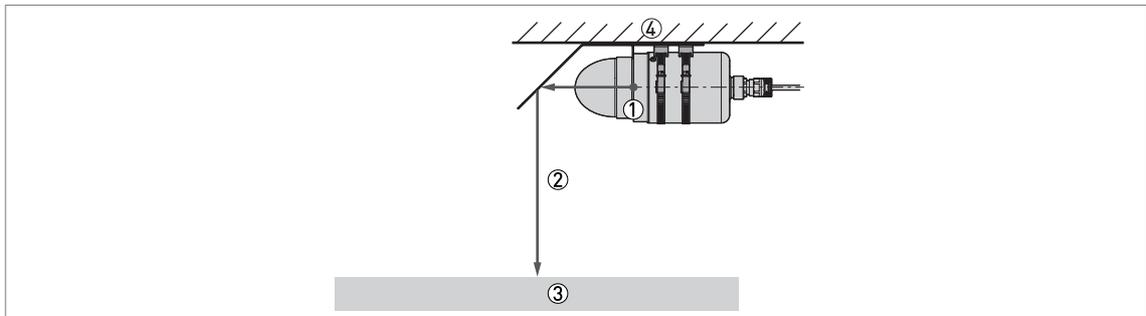
Figure 6-18: How to measure distance with the 45° deflector plate option
