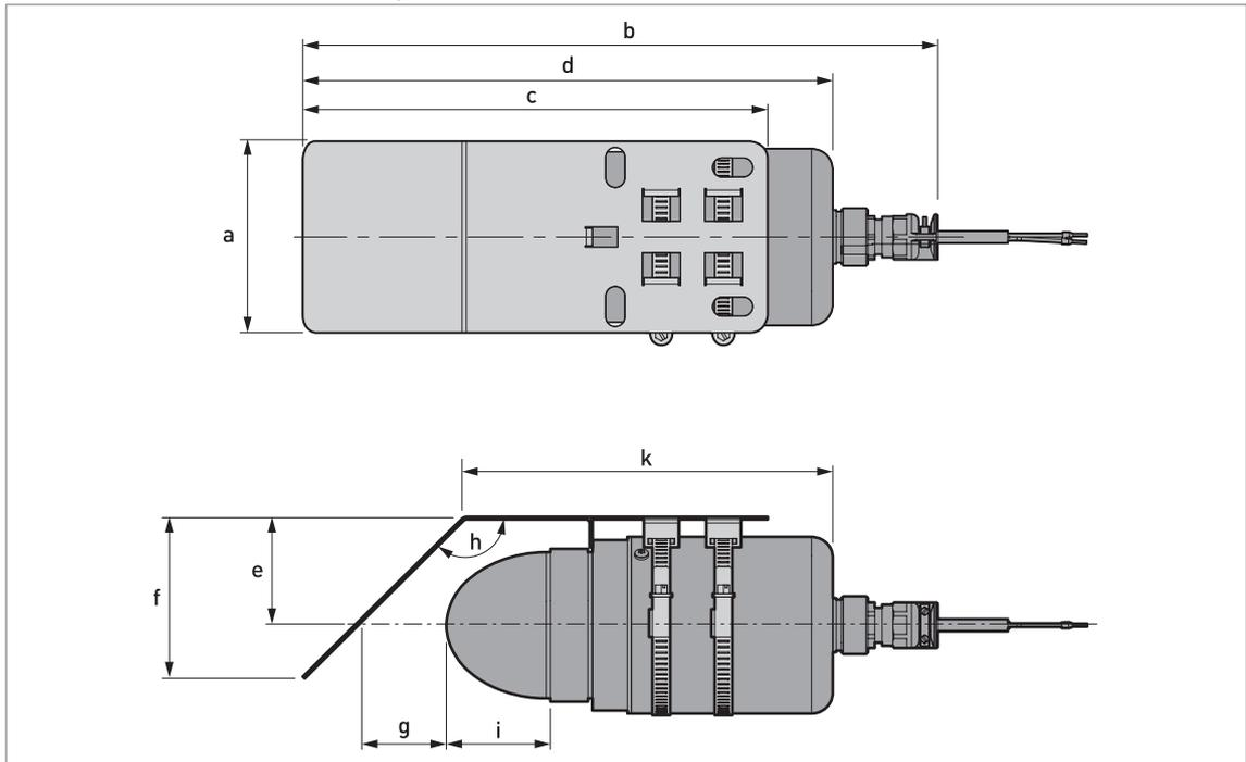
Figure 8-11: Device with a 45° deflector plate
