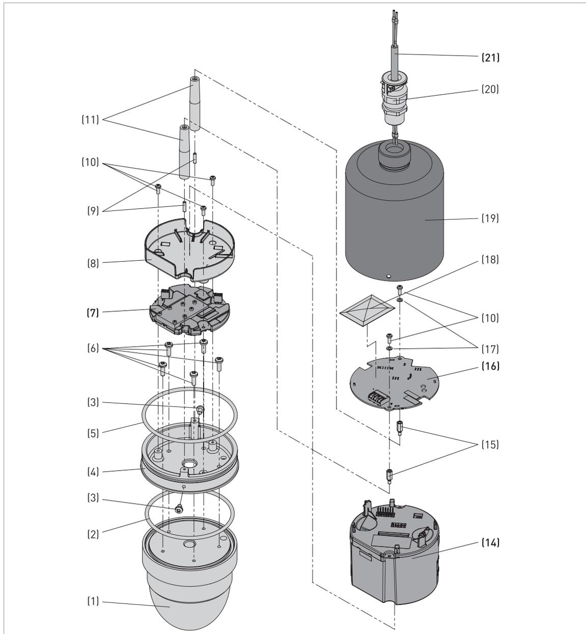
Figure 7-1: Parts of the device (refer to the "Parts list" table)
