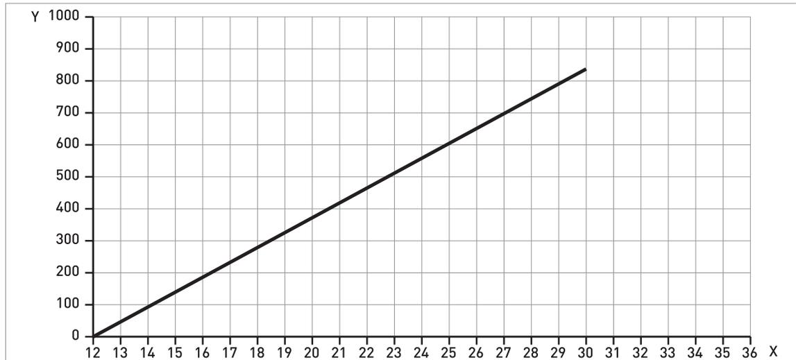
Figure 8-4: Minimum power supply voltage for an output of 21.5 mA at the terminals
