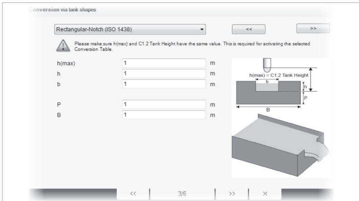
Figure 6-17: How to prepare a strapping table to measure volumetric flow rate in a flow channel
