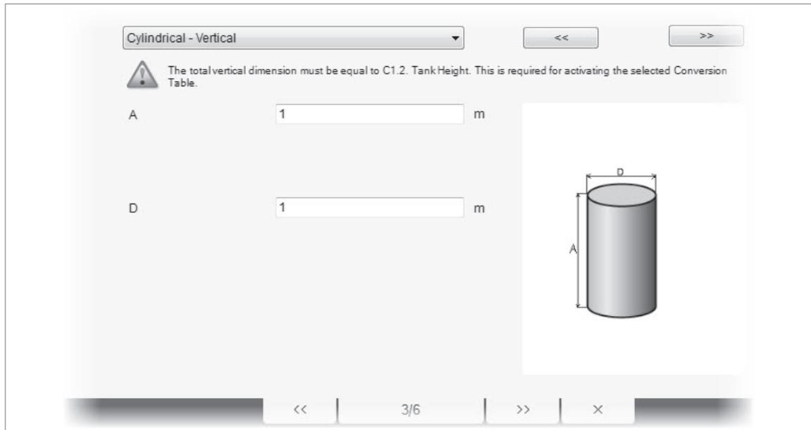
Figure 6-16: How to prepare a strapping table to measure volume in a tank
