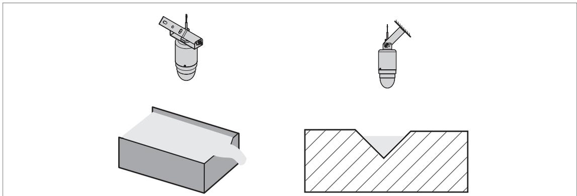
Figure 3-4: Recommended mounting position above a flume or a weir (open-channel flow)
