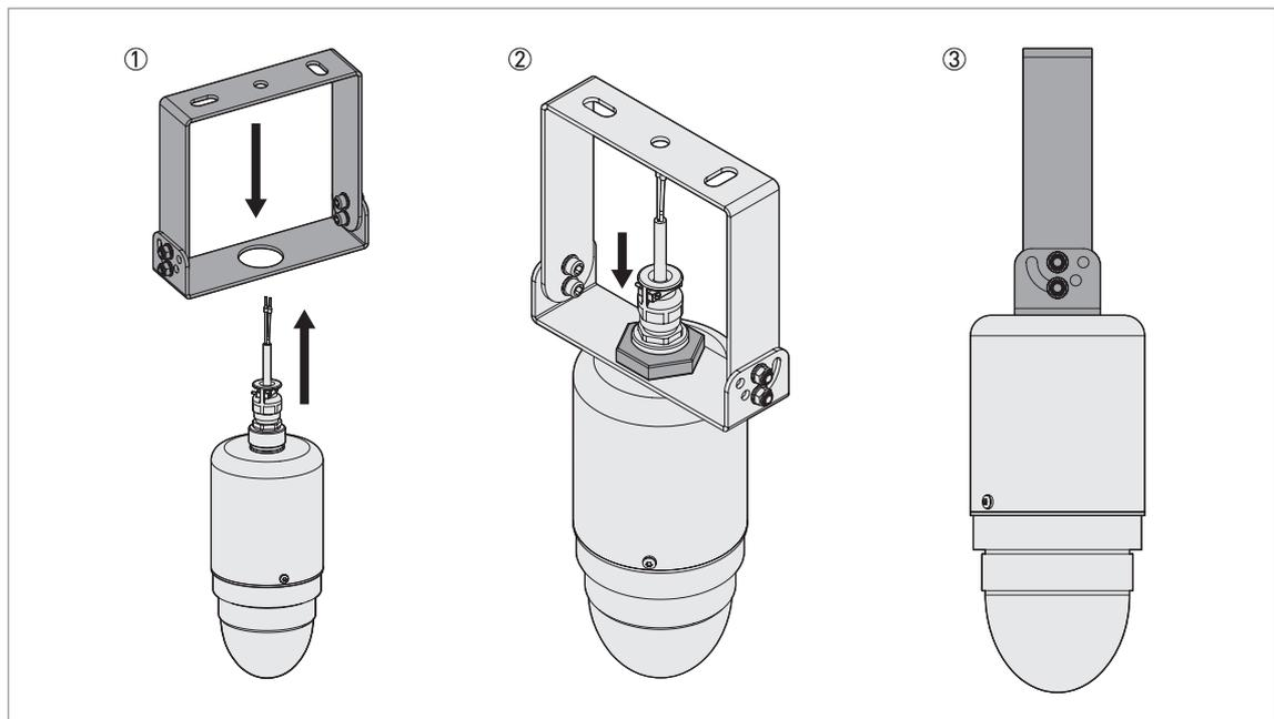
Figure 3-9: How to attach the orientable bracket to the device
