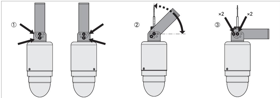
Figure 3-10: How to tilt the orientable bracket
