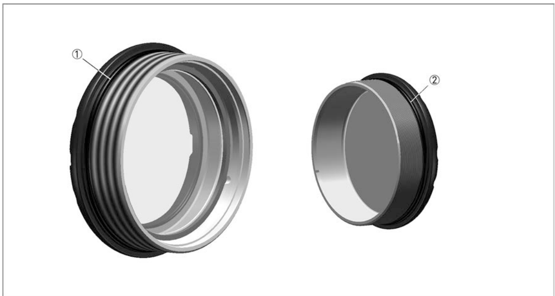
Figure 7-1: Maintenance of the O-rings
