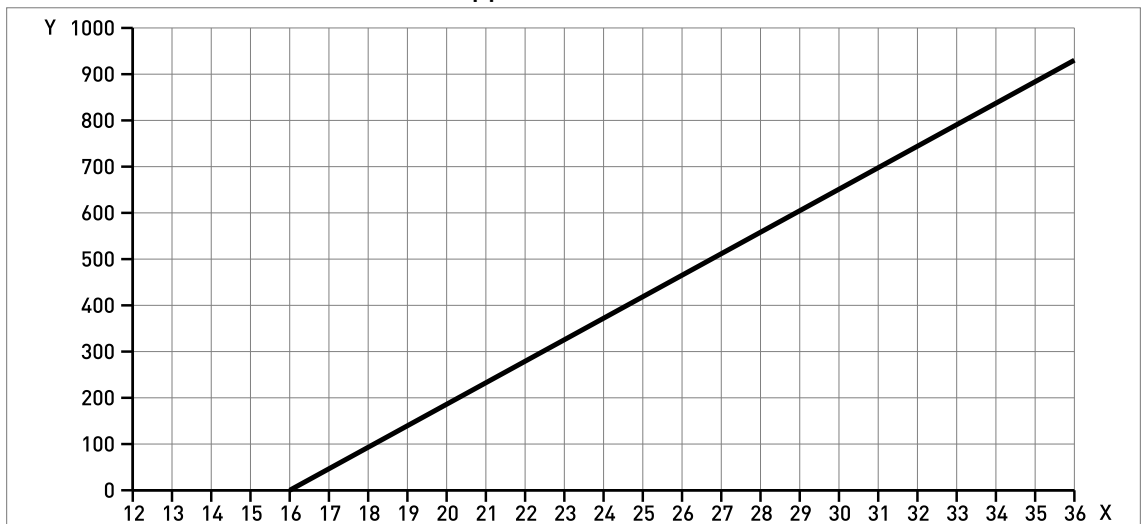
Figure 8-5: Minimum power supply voltage for an output of 21.5 mA at the terminals (Hazardous Location approval (Ex d / XP/NI))
