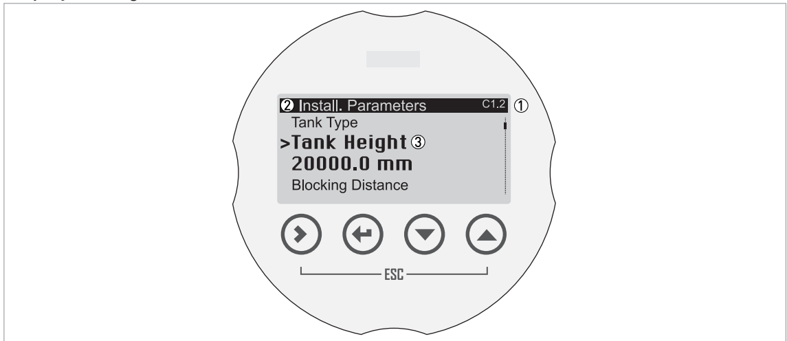
Figure 5-2: Display screen layout in Program mode
