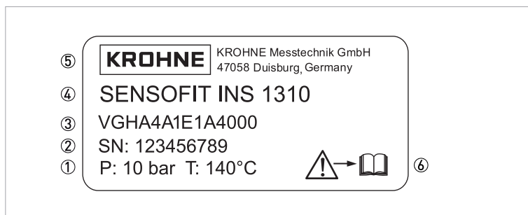
Figure 2-4: Example for a nameplate on the assembly body
