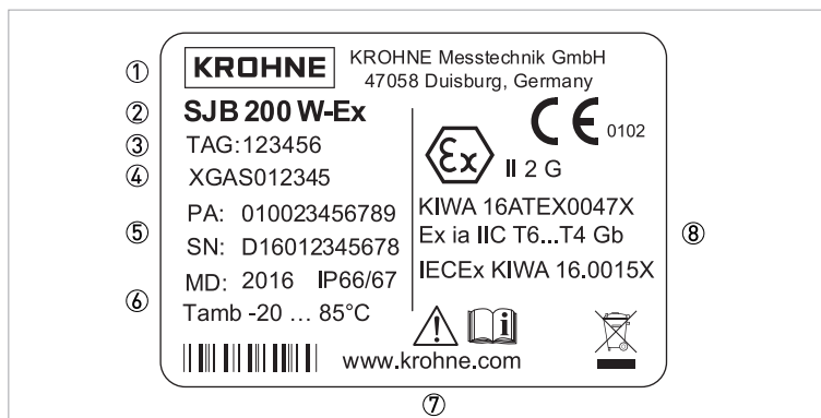
Figure 2-3: Example of a nameplate (ATEX) on the junction box
