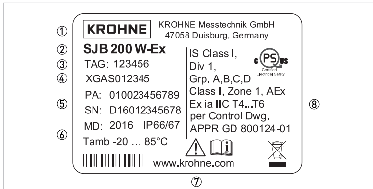
Figure 2-4: Example of a nameplate (QPS) on the junction box
