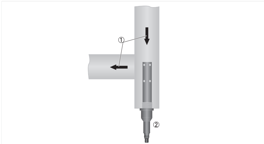
Figure 4-5: Installation for clean water
