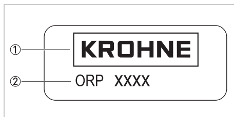
Figure 2-4: Example for a nameplate on the glass shaft
