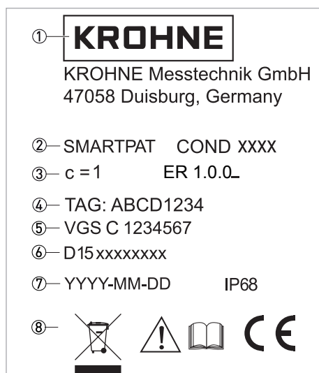
Figure 2-3: Example for a nameplate on the sensor body
